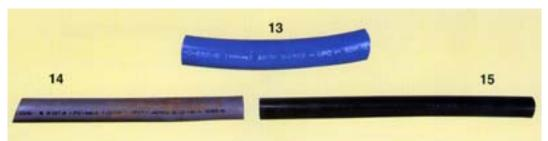
Polybutylene Pipe- Yard Service Line is typically blue (13), gray (14), or black (15). Inside Pipe is typically gray (14) or Black (15). Not that polybutylene pipe marked "PB 2110 M" is excluded.
